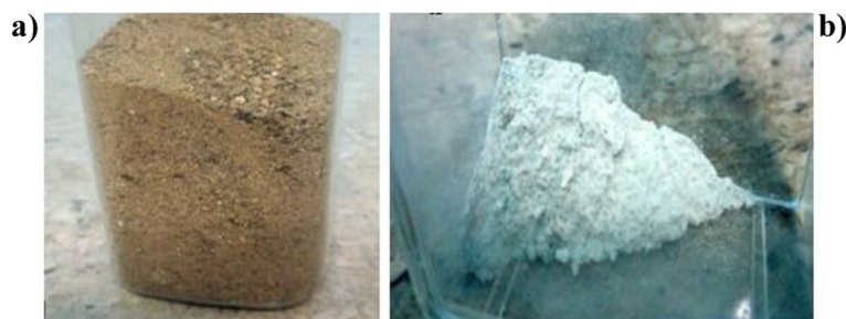
Fig. 5 Nendran banana peel powder a) before calcination b) after calcination at 700 °C
